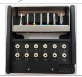
Drill stops are designed to precisely control osteotomy size by reducing the depth to which the bur can be inserted into the bone. Drill Stops are available as part of a set, with incremental (1.0mm) drilling depth reduction between 5.0 and 16.0mm. Thus a Drill Stop A (IN-DSC-05A) will reduce the maximum drilling depth of a bur by 5.0mm; Drill Stop B (IN-DSC-06A) by 6.0mm, etc.
